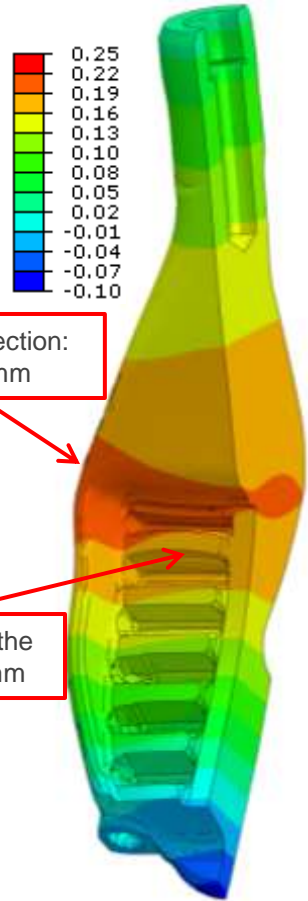
Horizontal deflection x100 (Scale: -0.1 → 0.25 mm)
