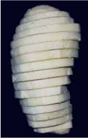
Polystyren mould (based on MRI previous segmentation)
